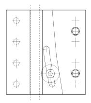
The safety gear must be mounted in pairs. They should be recessed into the structure, otherwise a limit stop shall be provided.
