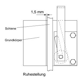
The knurled braking roller shall be in full contact with the guide rail blade.
